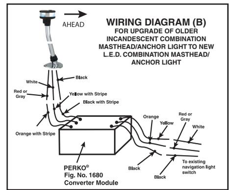
Attach supply connections to the light making sure to wire in accordance with both A.B.Y.C. Standard E11\* and U.S. Coast Guard Safety Standards for Boat Electrical Systems (33 CFR 183)\*. The supply leads are coded as follows:
